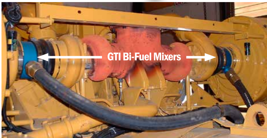
Typical GTI Bi-Fuel System Mixer Installation
